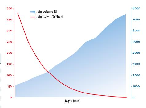
In combination with soil type, the critical value (max. value for infiltration system dimensions) could lie between 5 minutes (good soil) and 4320 minutes (clay or loam).
