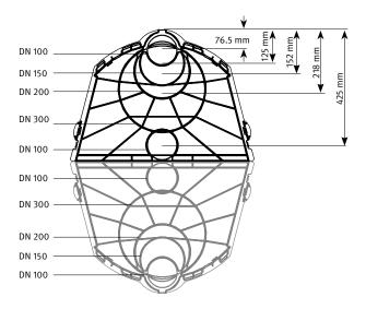
Infiltration Tunnel twin consisting of two identical Infiltration Tunnel half shells
